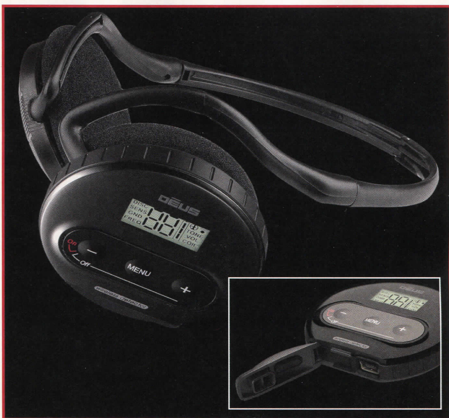
All of the electronics, including the digital LCD display, are encapsulated in a weatherproof disc on one side of the XP headset. Inset: USB connector.
