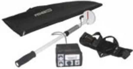
The Fisher M-101 metal detector was designed specifically for finding reinforcing bars and other metal objects embedded in concrete, conduits, PK nails, wiring, wall studs and other metallic objects. Users may expect accuracy to 1/4" of the centerline of the rebar.
